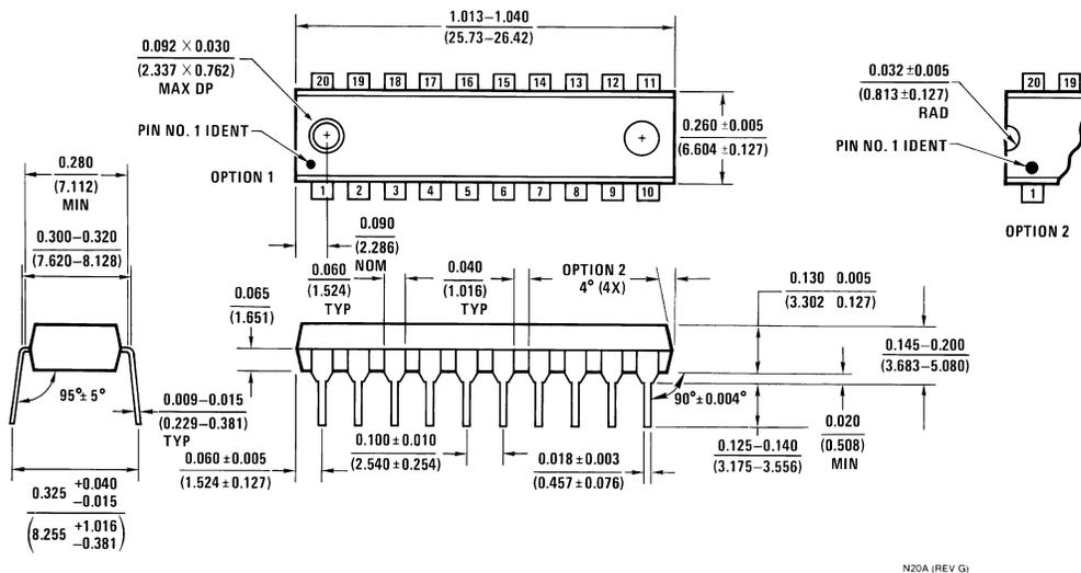
**20-Lead Molded Dual-In-Line Package (N)**
